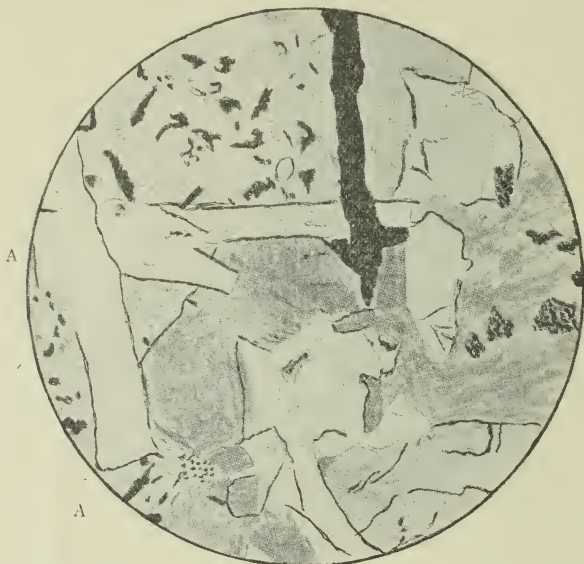
Figure illustrating original cavities in a rock of the copper bearing series such as may have been originally filled with chlorine gases, as at "A" wedged in between feldspar belts and an octagonal augite grain.
